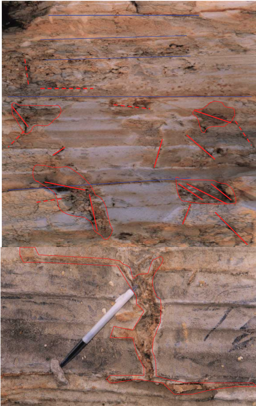
Figure 3.23: Intense oxidation developed around preferential flow paths. Blue lines = bedding planes, red solid lines = pre/syn oxidation processes, broken red lines = post oxidation cracks
