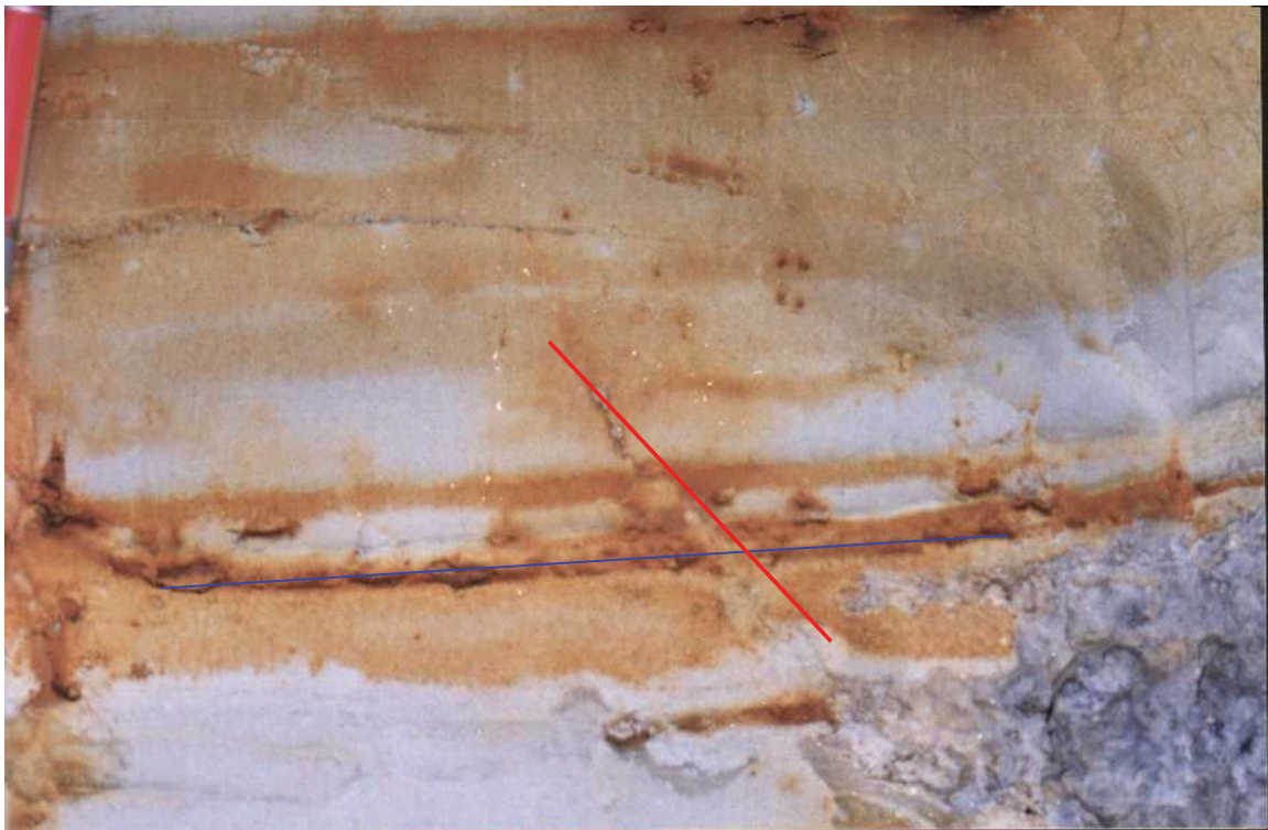
Figure 3.24: Bedding parallel oxidation. Note the bedding/fracture intersection
